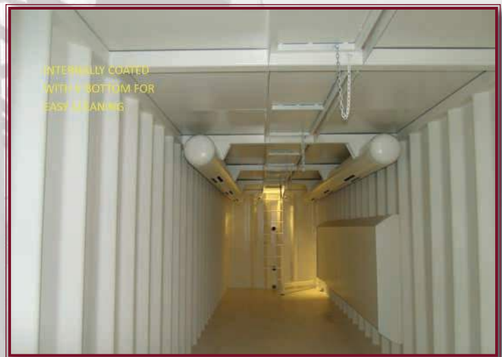
Twin 12" x 20' barrels with slotted bottoms on a 15 degree inward axis.
